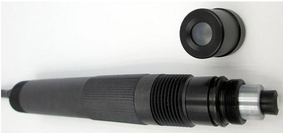
*Disassembled galvanic DO measuring cell ready for rebuilding. Cathode & anode on front tip of sensor are shown to the bottom right. High stability thick membrane installed into cap is shown immediately above. Membrane & electrolyte solution are easily replaced in just minutes when required. There is a virtually unlimited sensor lifetime achieved with this rebuildable type galvanic DO cell ensuring a very low total cost of ownership.*
