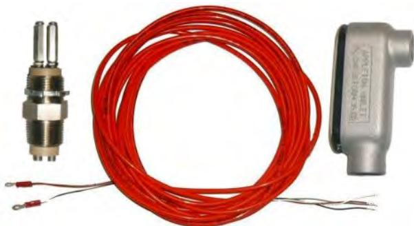
The SR2, 2 electrode sensor with conduit elbow and 20 foot cable. The SR2 is used for monitoring conductivity in a boiler blowdown line.
