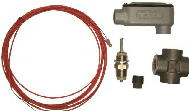
The SR2, 2 electrode sensor with conduit elbow, 20 foot cable, and ¾" cross. The SR2 is used for monitoring conductivity in a boiler blowdown line.
